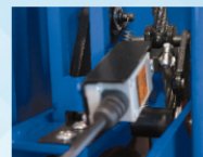
Limit switch sensor to confirm wire condition.
